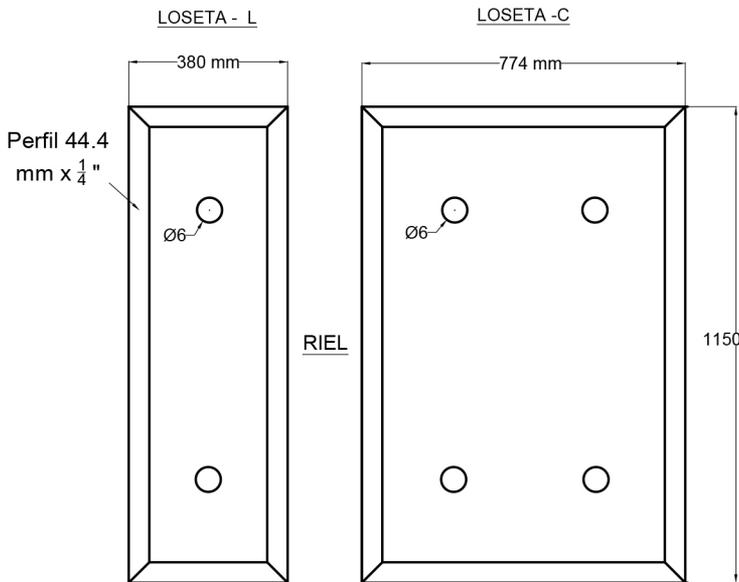
CORTE A-A' - LOSAS PASO NIVEL L - C
